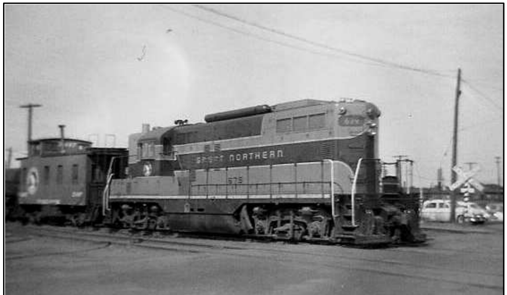
BNSF pre-merger GREATNORTHERN GP-7 roadswitcher No. 675 along with a wood-sided caboose making up a train in the Belknap St. Superior, WI yard in 1958.
