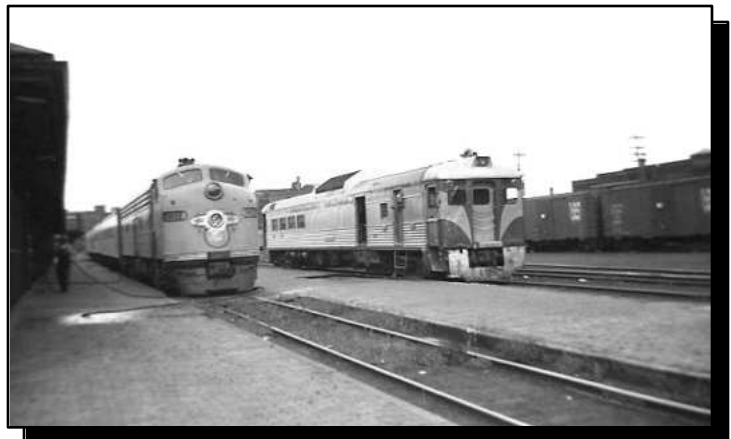
Short CN&W train behind single E unit, alongside Duluth Winnipeg & Pacific RDC-3 with its green & yellow striped nose. Note track weeds.
