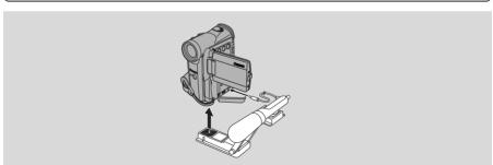
For greater creative control over audio recording, you can connect an external microphone to the camcorder via the MIC terminal. When using the MIC terminal, use a microphone with a built-in power supply (condenser microphone). It is possible to connect almost any stereo microphone with a plug diameter of ½ inch (3.5 mm), however, their audio levels will be different from that of the built-in microphone.
